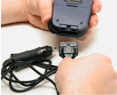
Attach external power cable to iFINDER.
